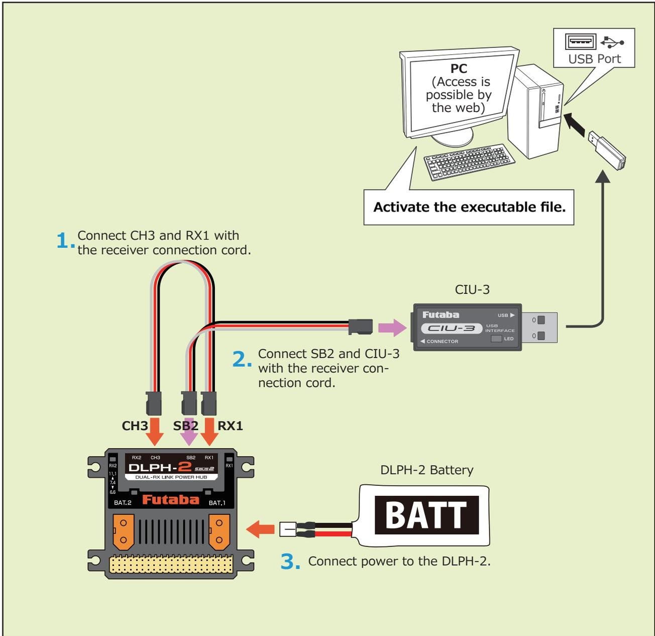
**4. Connect power to the DLPH-2, the RX1 and RX2 LEDs will light up green.**
