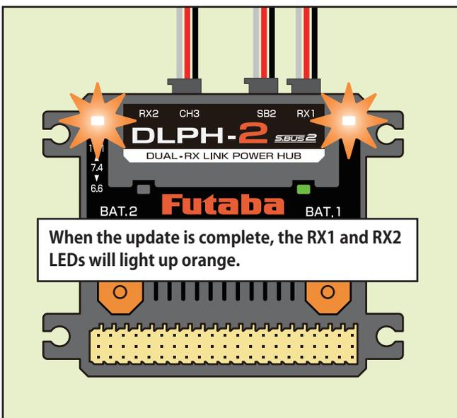
When the update is complete, the RX1 and RX2 LEDs will light up orange.
