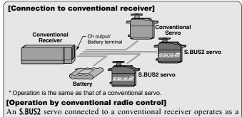
conventional servo. The channel becomes the receiver connection point. \*The contents set by programmable function are effective
