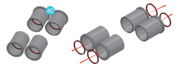
The piston ring and cylinder liner shall be matched one by one, and the corresponding cylinder liner
