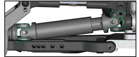
Correct driveshaft U-joint alignment.
